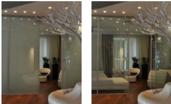
Smart glass will be used on the double-sided fireplace which switches from transparent to opaque for privacy between the living area and bedroom.
